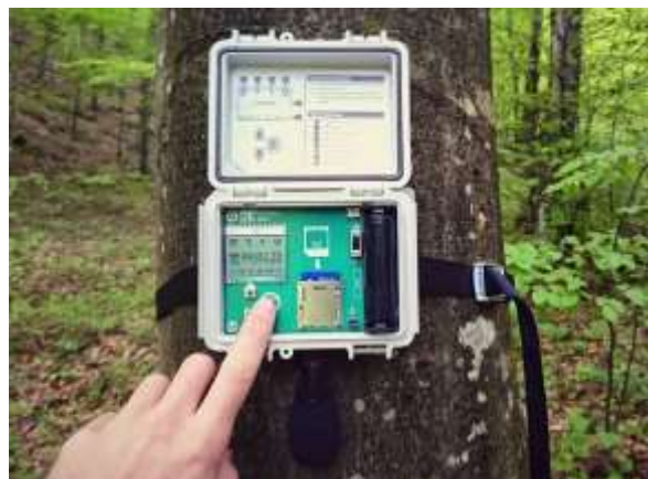
Bioacoustic audio recorder de Frontier labs. Source : http://www.frontierlabs.com.au/
